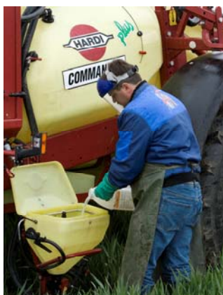
Induction hopper fixed to the sprayer (Source: DAAS, Jens Tønnesen)
