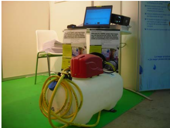
Clean water tank with a spray lance for external cleaning of the sprayer (Source: UPC)
